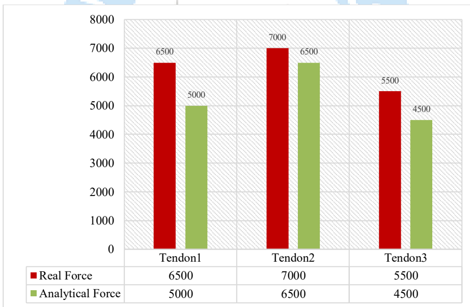
Fig 13: Comparison diagram of real and analytical prestressing forces, applying 20% Measurement error
