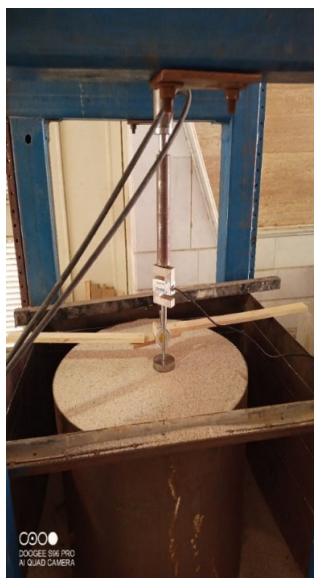
Fig 3. Circular foundation physical model system detail
