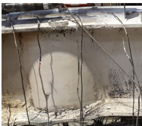
7% story drift in SW-RBS specimen
