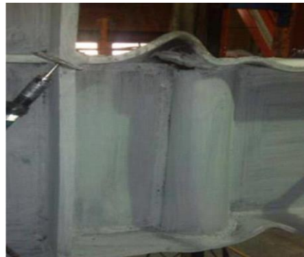
(b) 6% story drift in TW-RBS specimen
