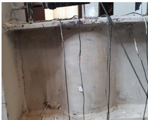
(a) 5% story drift in TW-RBS specimen
