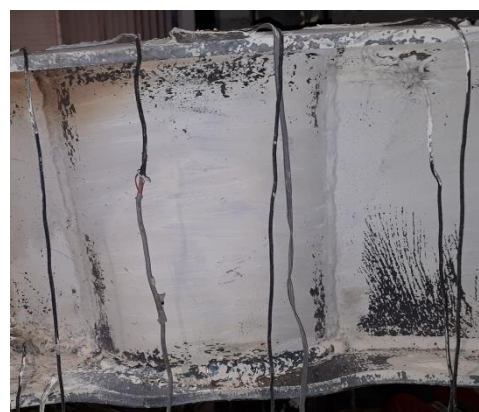
8% story drift in SW-RBS specimen
