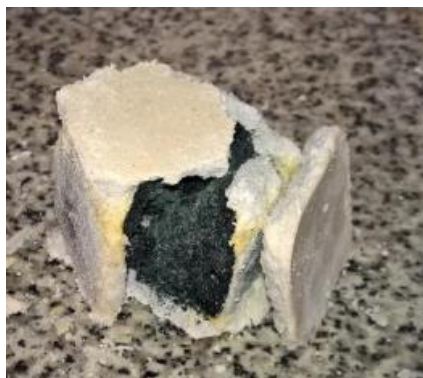
Figure 10. An example of Outer surfaces and inner parts of an AASP mortar specimen immersed in sulphuric acid after 91 days.
